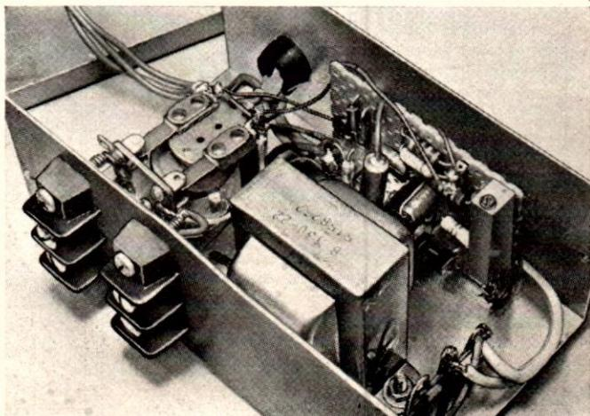
damage to these components. Use a low-wattage soldering iron, and apply the heat only long enough to get the solder to flow, while protecting the component lead with a heat sink. Also, make sure that electrolytic capacitors, diodes, and transistors are installed in the proper lead orientation.
